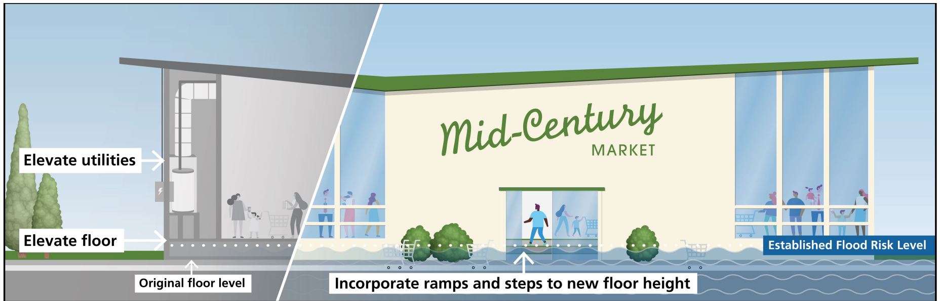
[100] Elevating the interior floor level above the established flood risk requires several building alterations, including constructing a new floor, elevating any utilities, and creating access to the new floor level. The original floor to ceiling height must be substantial enough to allow space for the new elevated first floor. Graphic: Blank Space LLC for NPS
