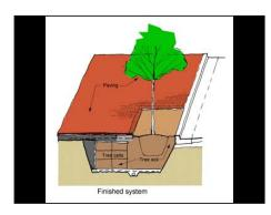
Then you can pave over the deck with any kind of paving you want as the deck is designed to take the water loading. If this was a porous pavement the water would go right down into the soil. Now do you really want to do that?
