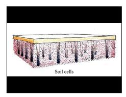
We're actually developing a box that we call a soil cell that will hold up a garbage truck while it's driving over. The pavement will give us 90% void space in the area that we can impact.
