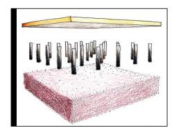
We would get more soil in less space and to do that we have to separate out the structure that holds up the sidewalk, from the soil that is supporting the tree. Could we design some kind of a system COVER
