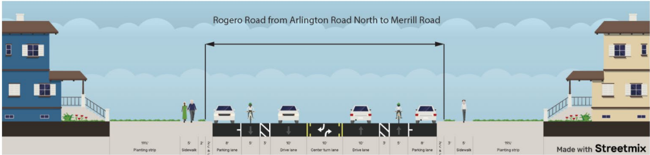
The lane repurposing concept includes buffered bike lanes and a two-way left turn lane. (Image: City of Jacksonville Planning and Development Department)
