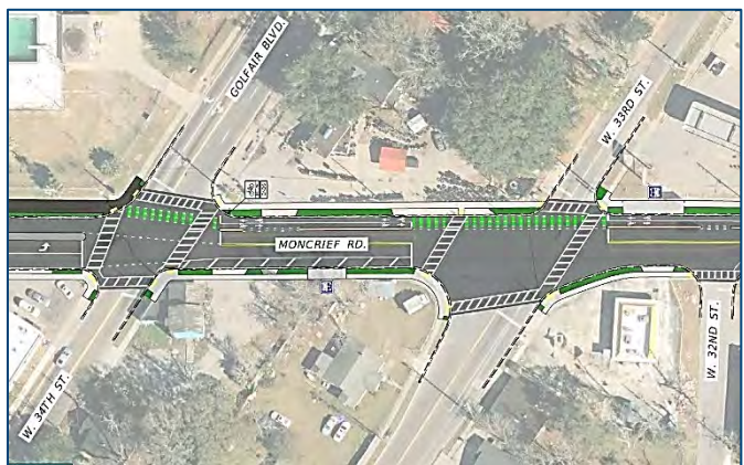
The segment between Golfair Boulevard and W. 33 rd Street serves as a transition between the adjacent three and four-lane existing typical sections.
