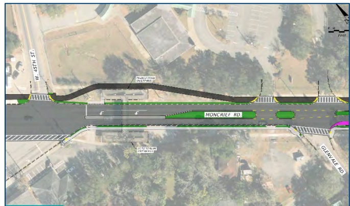
The shared use path will encroach minimally into Duval County School Board property at the pedestrian overpass ramp.
