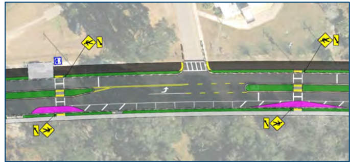
Midblock pedestrian crossings are provided between George R. Kerns Boulevard and Glenvale Road, all of which utilize the center median for pedestrian refuge.
