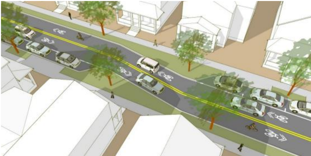
Figure 26: Residential Street Mid-Block Chicane Concept #9
