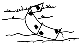
TYPE IV SILT FENCE
