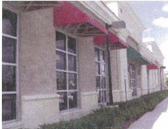
Figure 3: Pedestrian-scale facade with fenestration covering a minimum of 40% and maximum of 80% of occupant's linear frontage
