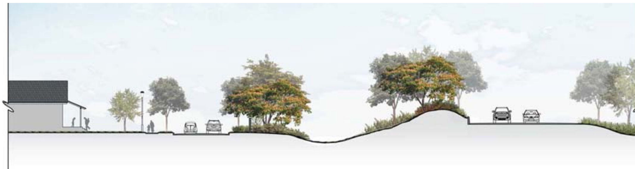
Section Illustration: The drawing above illustrates potential improvements to State Road 9A employing natural buffers. (Source: Zyscovich Architects, 2009)
