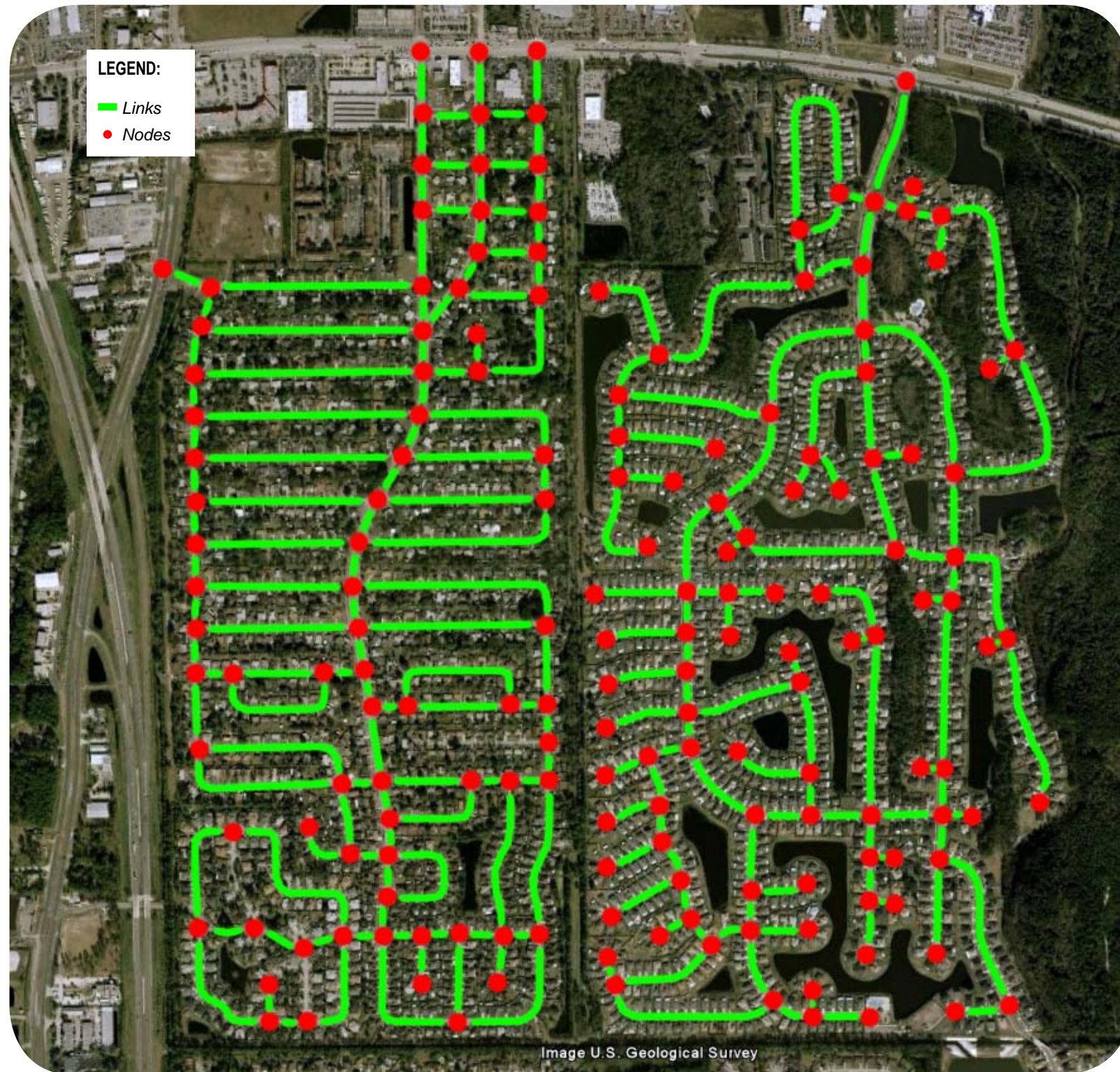
Diagram: Above is a connectivity index comparison of two residential subdivisions in the District. On the left, the connectivity index is 111 links/76 nodes = 1.46. On the right, the connectivity index is 101 links/95 nodes = 0.94. Minimum standards for connectivity index typically range from 1.2 to 1.4. (Source: Zyscovich Architects, 2009)
