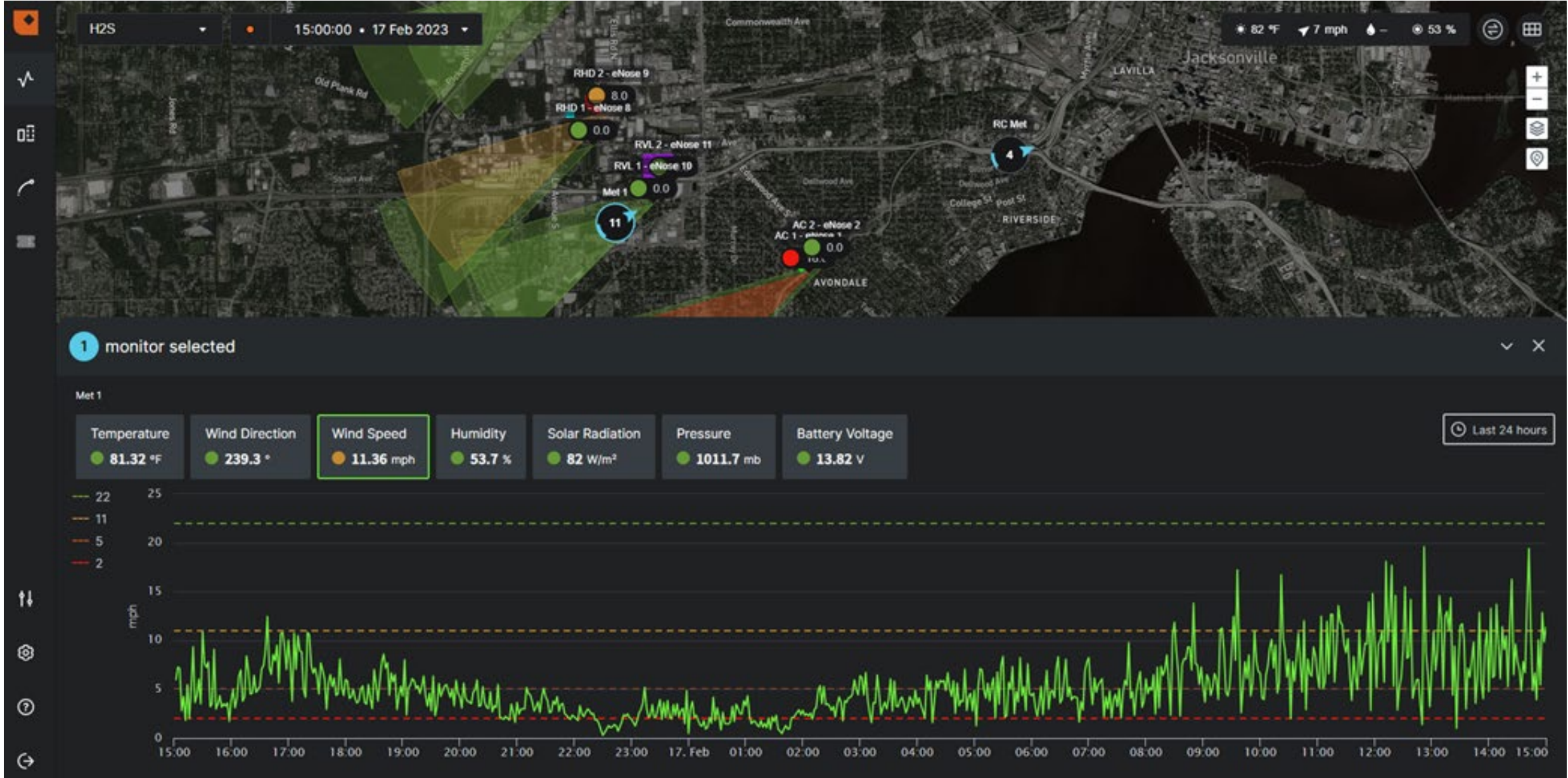
Figure 17. Monitoring Module feature to view past data for selected parameters.
