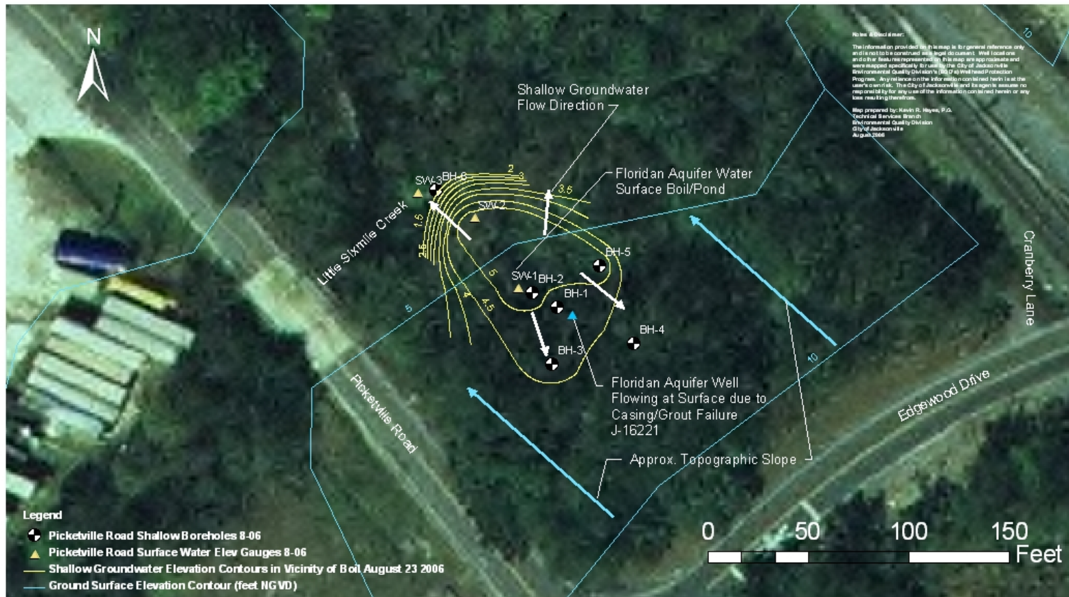
Influence of a Failed Flowing Well on the Shallow Water Table Picketville Road Area Well J-16221 August 2006
